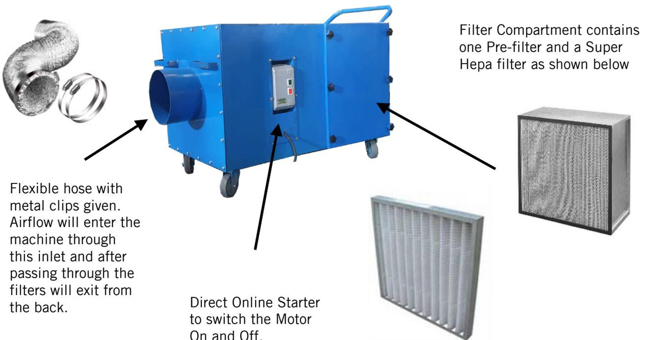
Flexible hose with metal clips given. Airflow will enter the machine through this inlet and after passing through the filters will exit from the back.
